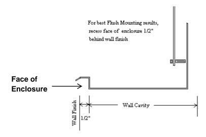
For best **Flush** Mounting results, recess face of enclosure's lip
